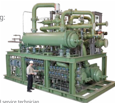
A field service technician evaluates instrument readings on a 5-stage MSG-3 carbon monoxide compressor.
