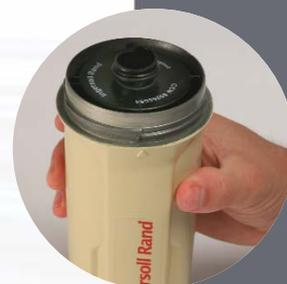
3. To install a new element, simply place it into the bowl and screw the bowl back to the head of the filter body.
