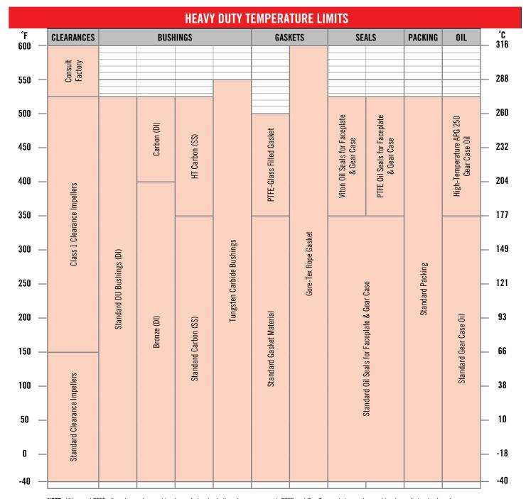
**NOTE:** Viton and PTFE oil seals can be used in place of standard oil seals upon request. PTFE and Gor-Tex gaskets can be used in place of standard seals upon request. If using a mechanical seal, please consult factory for temperature limitations.
