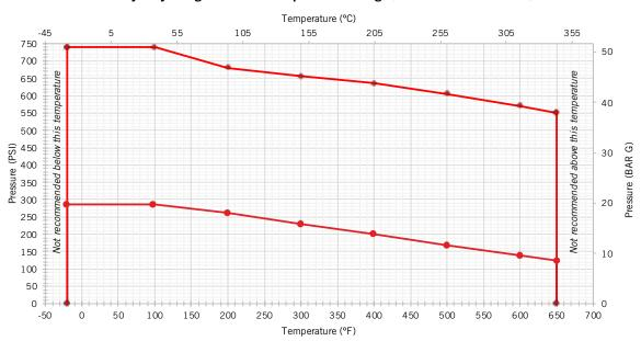
**NOTE:** These charts show ratings for the flanges only. The maximum pump operating conditions must be considered. Consult the appropriate catalog for the maximum allowable pressure and temperatures. These ratings are non-shock pressure.
