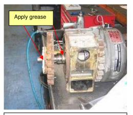
15. Apply some grease to inside of shaft seal in side plate & shaft. Push side plate over shaft taking care not to damage the seal.
