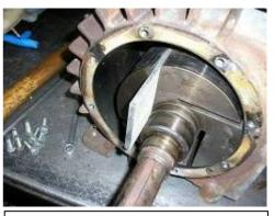
11. Lightly oil blades on both sides using a clean paint brush
