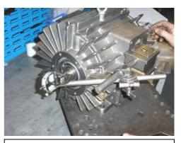
18. Add clock (DTI) to m/c and check end float. (If not correct as per specification it will then be necessary to remove side plate and repeat steps 13-18)
