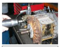
17. Secure side plate to body using(8) cap screws. Check to see ifmachine runs free by rotating shaft
