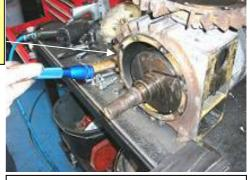
10. Check rotor & inside of body to ensure there are no blades or debris remaining (blow out using an airline)
