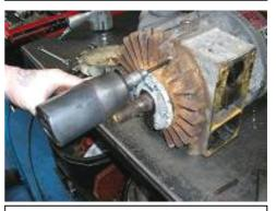
6. Remove (6) cap screws from side plate
