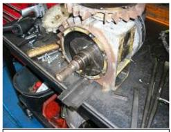
9. Remove old blades from rotor. (rotating the rotor helps when removing the blades)
