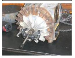
3. Carefully remove fan using a set of pullers as shown (or tap from the rear using a blunt chisel or screwdriver)
