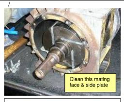
13. If shim is damaged, remove & clean body & side plate mating surfaces. Measure & note the shim thickness
