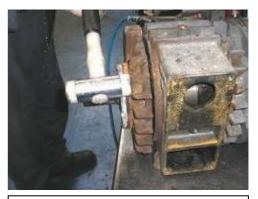
16. Tap side plate & locate into body using existing dowel pins
