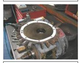
14. Obtain shim of same thickness as before. Lay over side plate and line up with dowl pins & holes.
