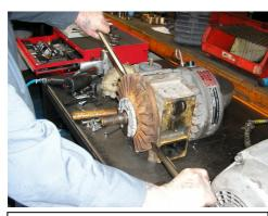
7. Carefully prise side plate from the body and remove.
