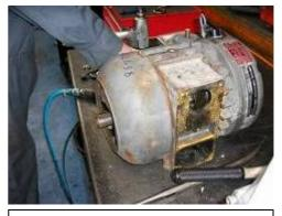
22. Re-fit cowl using (3) cap head screws. Ensure rotor runs freely. Also, ensure blades drop freely
