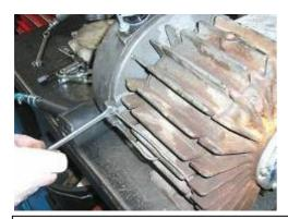
19. Re-attach oil pipe (blow through the oil pipes to ensure they are clear of any debris)
