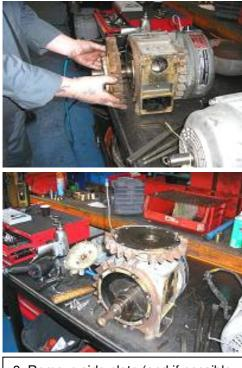
8. Remove side plate (and if possible gasket) to expose rotor & blades
