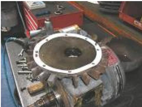
14. Obtain shim of same thickness as before. Lay over side plate and line up with dowl pins & holes.
