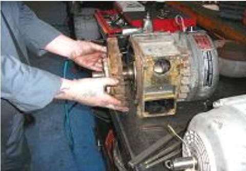
8. Remove side plate (and if possible gasket) to expose rotor & blades
