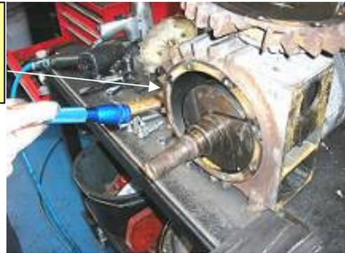
10. Check rotor & inside of body to ensure there are no blades or debris remaining (blow out using an airline)
