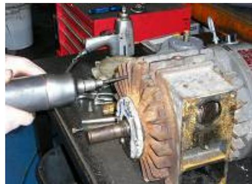
17. Secure side plate to body using (8) cap screws. Check to see if machine runs free by rotating shaft
