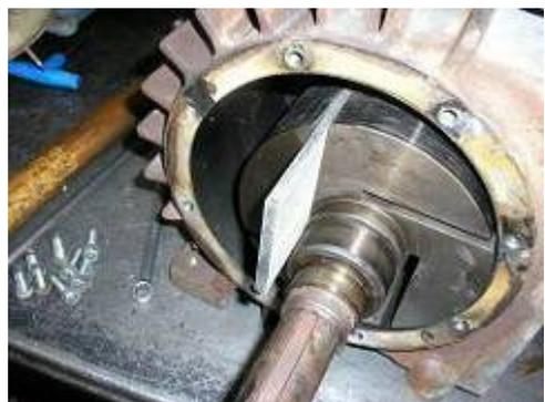
11. Lightly oil blades on both sides using a clean paint brush
