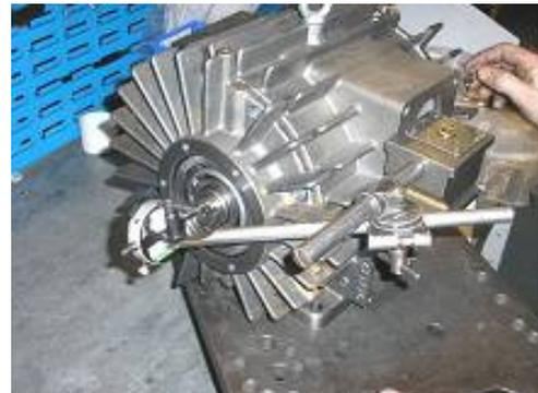
18. Add clock (DTI) to m/c and check end float. (If not correct as per specification it will then be necessary to remove side plate and repeat steps 13-18)
