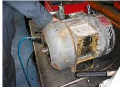
22. Re-fit cowl using (3) cap head screws. Ensure rotor runs freely. Also, ensure blades drop freely
