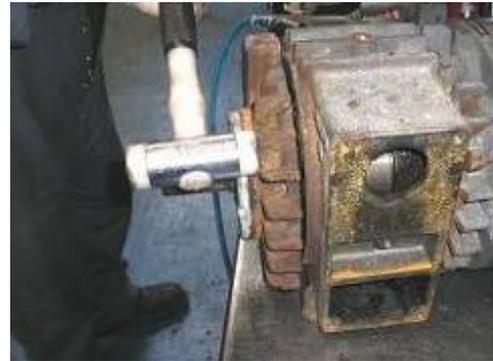
16. Tap side plate & locate into body using existing dowel pins
