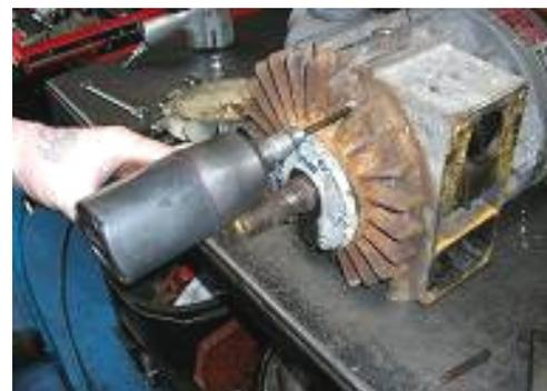
6. Remove (6) cap screws from side plate
