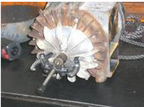
3. Carefully remove fan using a set of pullers as shown (or tap from the rear using a blunt chisel or screwdriver)
