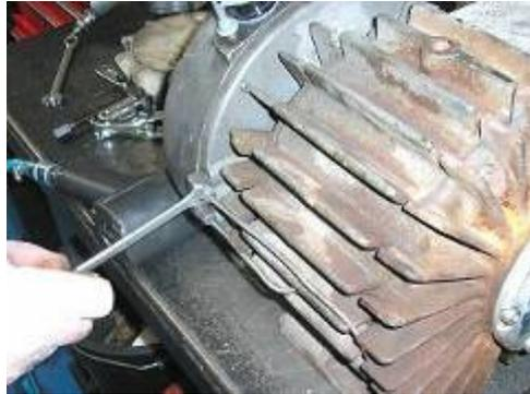
19. Re-attach oil pipe (blow through the oil pipes to ensure they are clear of any debris)
