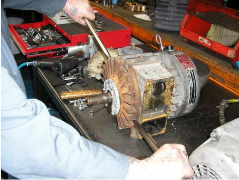
7. Carefully prise side plate from the body and remove.
