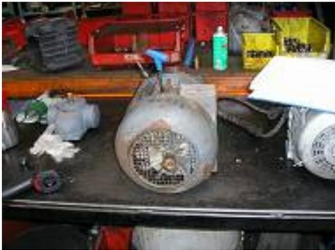
1. Remove (3) cap head screws from the drive end fan cowl
