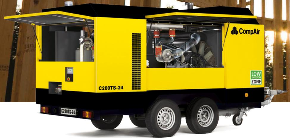
The TurboScrew compressor range with their unique patented twin-turbo diesel engines offer world class efficiency figures with a weight payload of 3,500 kg.
