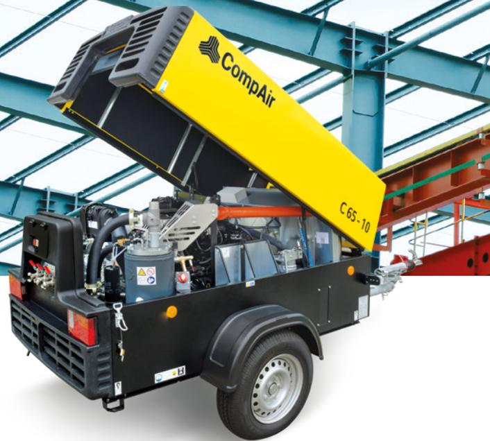
This new range of compressors stands out for its low diesel consumption, which is 10% less than the previous range. This is a mechanically controlled diesel engine without a particulate filter that meets the European Stage 3a emissions standard. Thanks to a wide pressure range up to 14 bar, this compact compressor range is extremely versatile and meets the requirements of numerous applications.
