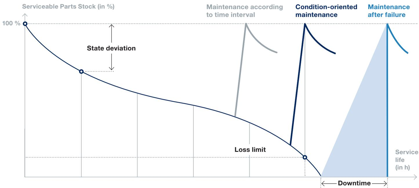
Fig. 3: Degradation curve of the degree of wear of a component
