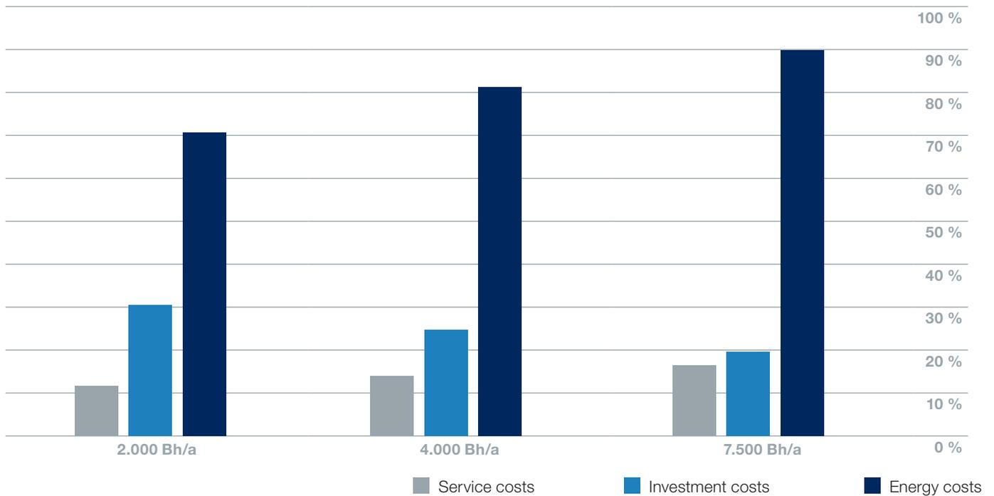
Fig. 1: Presentation of the cost distribution in the company using the example of a compressed air system
