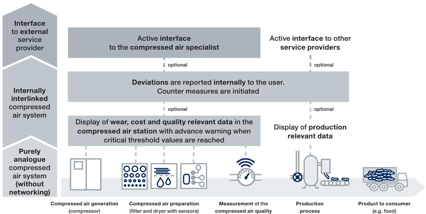
Fig. 2: Possibilities of networking using the example of a compressed air system
