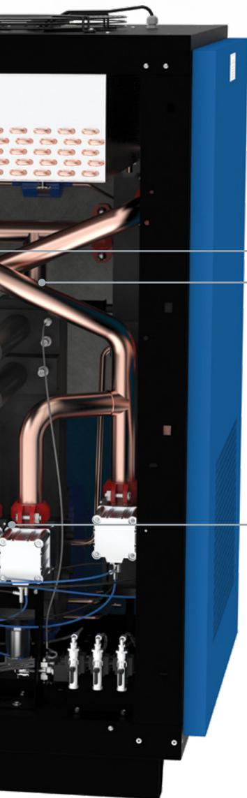
**DRYING:** With only 15% of the moisture remaining, the air now enters the sub zero dryer heat exchanger where it is cooled and dried to  $-20^{\circ}\text{C}$  ( $-4^{\circ}\text{F}$ ) PDP. The removed moisture begins to form a thin layer of frost on the inner walls of the heat exchanger.
