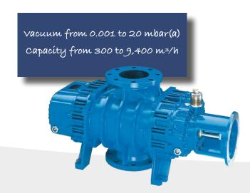
The RBS-AV series are rotary lobe blowers used to increase the capacity of the primary vacuum pumps when operating at their minimum suction pressure (as a booster).
