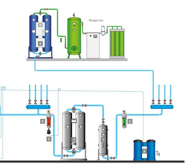
**5. Condensate drain:** Drains are needed at all separators, filters, dryers and receivers in order to remove the liquid condensate from the compressed airsystem.
