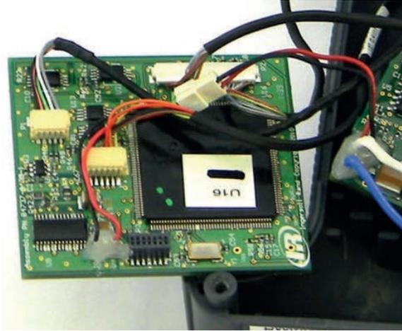
10. Connect the Hall Cable to its connector on the foot PCB, the transducer cable to its connection, and the connection between the foot PCB and the handle PCB.
