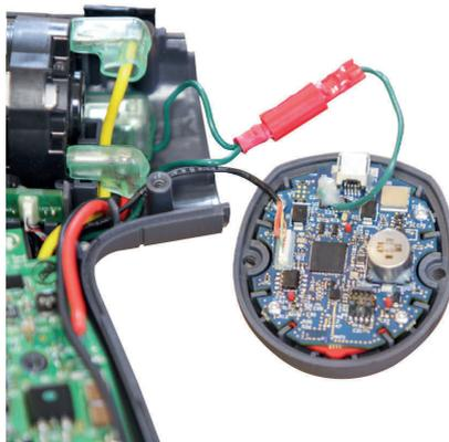
18. Connect the ground cable connector and the Interface cable connector to the display board.
