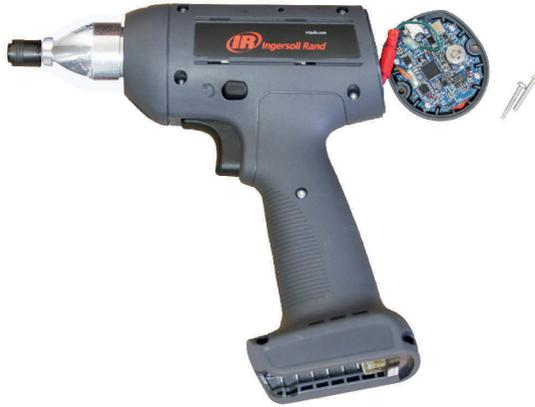
22. Install the backcap onto the housing and secure it with two screws tightened to 1 Nm.
