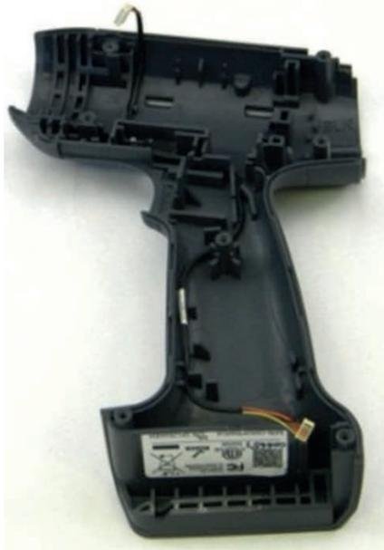
5. Route the hall cable through the housing following the shadow line, leaving approximately 1 1/2" of cable above the housing where the cable connects to the motor.
