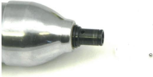
2. Then remove the ball from the spindle by inserting a punch or thin blade screwdriver into the hex of the spindle and pushing the ball out of its hole. Examine all parts for wear and damage.
