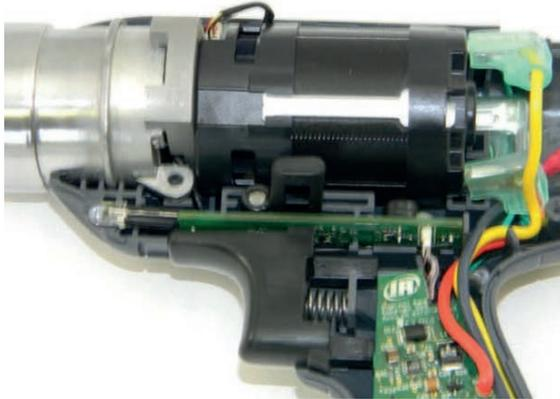
16. Install the trigger with the spring into the housing. Tilt the assembly at approximately a 45° angle with the rear down. Then slide the assembly into position. Also install reverse lever into the slot in the housing.
