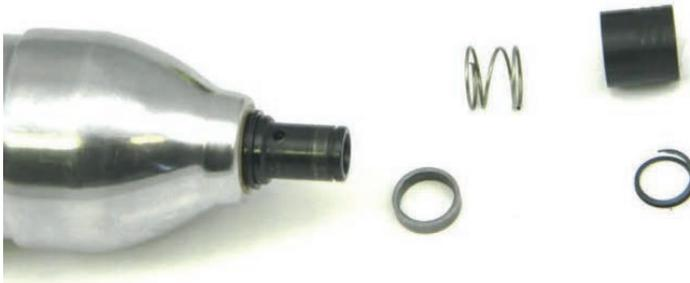
1. For units with the 1/4" quick change spindle, disassemble the spindle as follows. Remove the spiral spring clip from the front of the spindle, then remove the quick change collar, spring, spring support and rear spiral snap ring.
