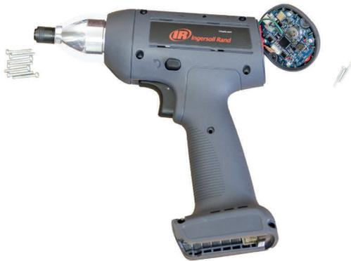
20. Gently lower the housing down onto the unit. Ensuring that all of the components and cables are in their proper position. Closing the tool by starting at the bottom at the foot PCB and working your way to the motor and the top of the tool.
