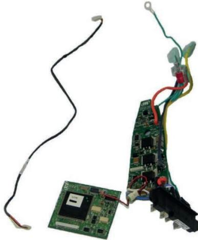
16. This will leave the Hall Cable which can now be disconnected from the foot board and the cable removed.
