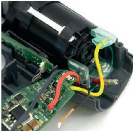
13. Connect the three motor leads, in their proper orientation. The black lead is connected to the bottom lug (closest to the housing). The yellow lead to the top lug, and the red lead to the middle lug (closest to the trigger board). There are also markings on the housing halves to aid in the orientation of these leads. Also ensure that the terminals are connected at the proper angle.
