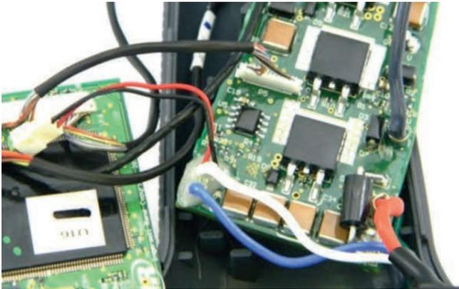
11. Connect the Interface cable to the handle PCB.
