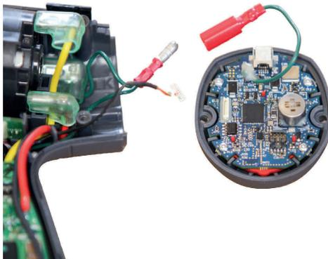
5. Disconnect the pin connector first, then disconnect the ground wire slip connector. Remove the USB port cover from its slot in the housing.
