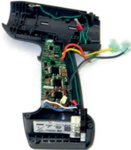
6. Route the green ground wire through the housing and to the top front screw lug.
