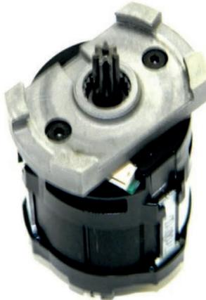
1. Install the motor mount onto the motor. Align the mount so that the slot in the mount is on the opposite side of the motor from the motor connector as shown in the photo. Torque the motor mount screws to 0.5 Nm.
