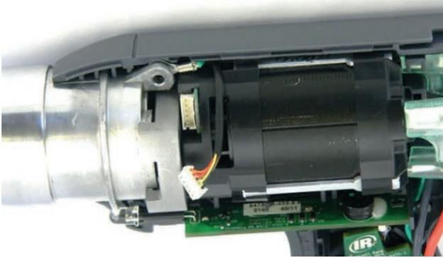
14. Connect the Hall Cable with its connector on the motor.
