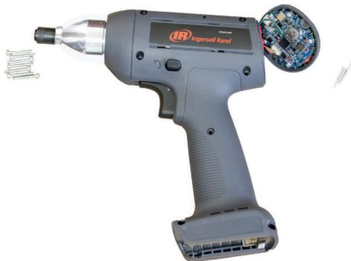
21. Install the housing screws in the tool to 1 Nm. Starting with the center screw, then the top two screws, proceeding to the middle and finishing with the bottom to screws.
