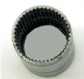
6. Inspect the ring gear for wear and damage.
