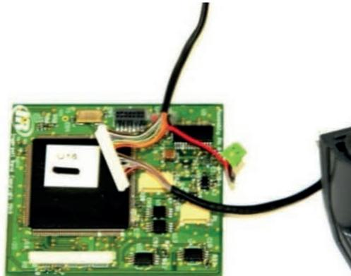
9. Connect the connector of the Interface cable to its connector on the foot PCB.
