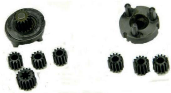
7. Disassemble the planetary gears and the pinion gear from the spindle assemblies. Inspect the gear teeth and shaft holes for wear and damage. A pinion gear is used on the 4 Nm and 8 Nm tools only.
