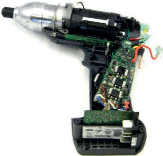
15. Install the Handle PCB onto the center screw lug. Ensure that the O-ring is in position on the lug underneath the board. Again ensure that all the cables are routed properly and fully seated.
