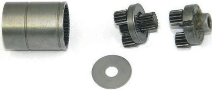
5. To disassemble the gear pack, slide the planetary gear spindles and the plate out of the ring gear.
