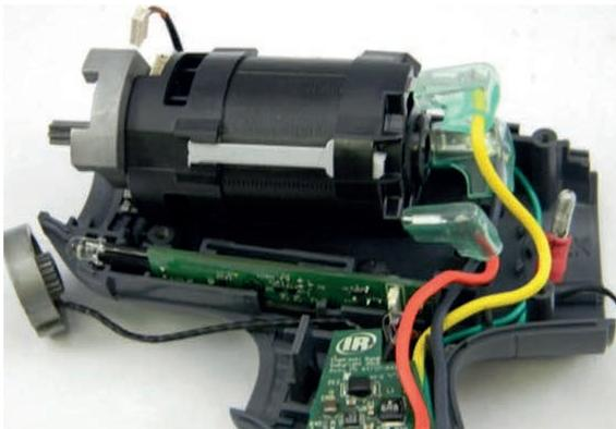
11. Unplug the three motor terminals from the rear of the motor, by pressing the locking detents on the connectors under the clear boots. Note the orientation of the three terminals. They must be installed in the same orientation when the tool is reassembled. Now remove the motor from the housing.
