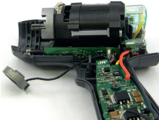
10. While tilting the motor up slightly, remove the transducer from the front of the motor.
