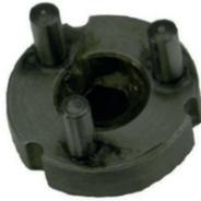
8. Also check the planetary spindle shafts for wear and damage. This completes the disassembly of the unit.
