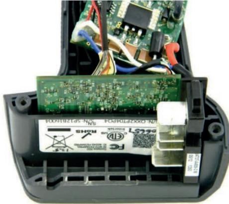
12. Install the foot PCB and the battery interface. Retrace and fully seat all the cables, ensuring that they are in their proper position. Also ensure that the trigger board is still in place. Any cables which are not seated properly will be damaged resulting in the tool not performing properly.
