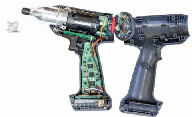
19. Install the second half of the housing onto the unit by tilting the bottom of the housing and align the housing and the foot PCB. Slightly push forward on the board to ensure it seats into the slots in the housing.
