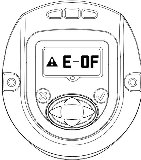
3. Check the tool's display for any error messages displayed on the screen. If the screen is dark, you will have to depress the trigger to wake up the tool.
