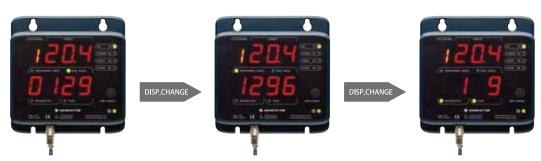
Display Upper row: Tool, work / Torque Lower row: Free running angle
