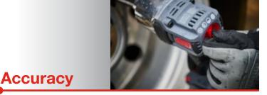
Versatile features enable reliable performance at every stage of tire maintenance. High breakaway torque, variable speed triggers, and advanced diagnostics tighten fasteners to exact specifications, reducing errors, improving accuracy, and avoiding repeated maintenance.
