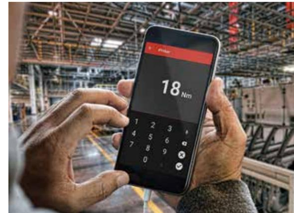
The INSIGHT™ Connect app will help you stay productive, mobile and in control of your fastening process. It programs any Ingersoll Rand® QX Connect Series™ tool without the need for additional technical training, special software, plant network permissions or a laptop computer. Working from a smartphone or tablet, operators can use the app to quickly program the torque and angle control configurations on these closed-loop, transducerized tools.
