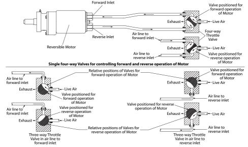
Two three-way Valves for controlling forward and reverse operation of Motor
