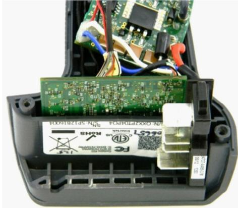
12. Install the foot PCB and the battery interface. Retrace and fully seat all the cables, ensuring that they are in their proper position. Also ensure that the trigger board is still in place. Any cables that are not seated properly will be damaged resulting in the tool not performing properly.
