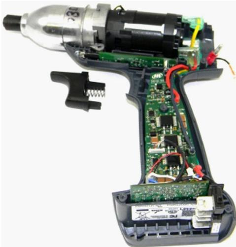
6. Remove the trigger by pulling the trigger up slightly and out of the housing. Also remove the reverse lever from the housing.
