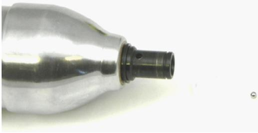
2. Then remove the ball from the spindle by inserting a punch or thin blade screwdriver into the hex of the spindle and pushing the ball out of its hole. Examine all parts for wear and damage.
