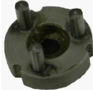
8. Also check the planetary spindle shafts for wear and damage. This completes the disassembly of the unit.
