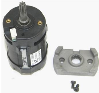
12. Using a 2mm Allen wrench, remove the two Allen Screws which hold the motor mount onto the motor. Then remove the mount.
