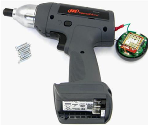
21. Install the housing screws in the tool to 1 Nm. Starting with the center screw, then the top two screws, proceeding to the middle and finishing with the bottom to screws.
