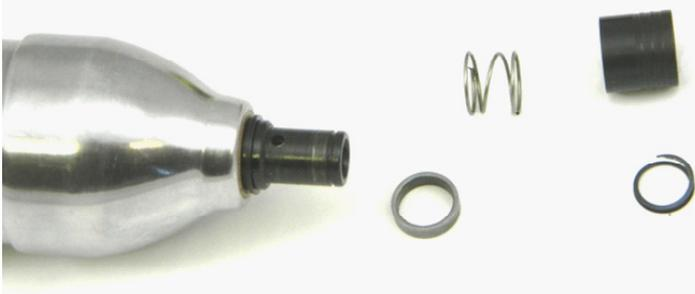
1. For units with the 1/4" quick change spindle, disassemble the spindle as follows. Remove the spiral spring clip from the front of the spindle, then remove the quick change collar, spring, spring support and rear spiral snap ring.
