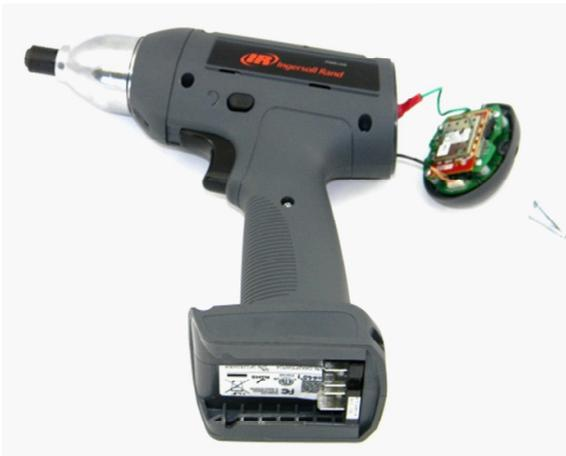
22. Install the backcap onto the housing and secure it with two screws tightened to 1 Nm.
