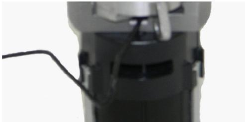
2. Install the transducer over the motor shaft and onto the motor. Be sure the transducer cable is on the center to left side of the notch of the motor mount. If the cable is not orientated in this way it will be damaged when the tool is reassembled.
