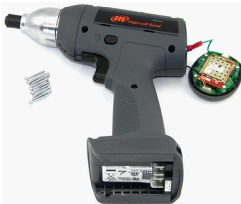
20. Gently lower the housing down onto the unit. Ensuring that all of the components and cables are in their proper position. Closing the tool by starting at the bottom at the foot PCB and working your way to the motor and the top of the tool.
