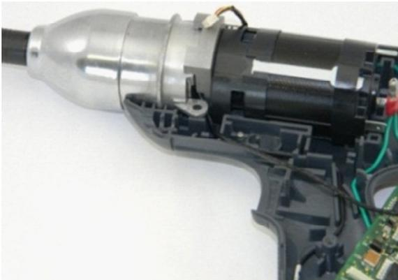
7. Install the motor/gear case assembly into the Housing. Seat the rear of the motor first then, carefully lower the assembly into position. Add a service loop to the transducer cable under the gear case ear. Ensure that all the cables are clear of the assembly and that they have not been pinched or cut. Also be sure that the assembly is fully seated in the housing.
