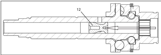
11. Grease 3 X cross holes of driver shaft with **Ingersoll Rand 40036-1** Grease and Insert 2 X Plunger Ball 2.38mm (19) Per Hole. See section view below for the proper placement.
