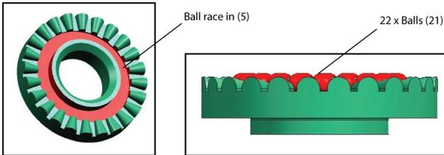
22. Thread Adjustment Nut (5) with balls in it onto Assembly of Step (20) and tightened with hand first.
