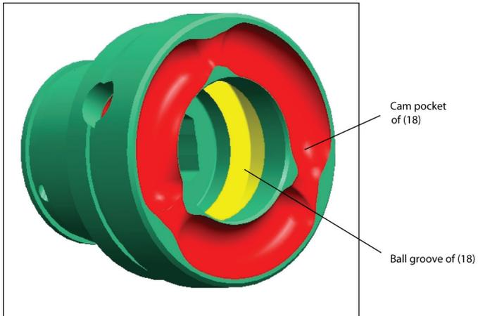
2. Fill Ball Groove and Plunger Hole of Driver Shaft (9) with **Ingersoll Rand # 40036-1 Grease**.
