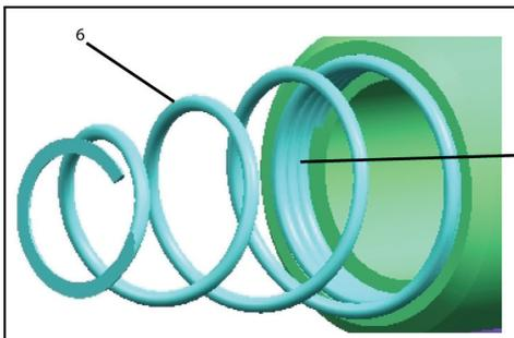
12. Align Ball Spring above Ball (5) and Thread into Throttle Housing (1).
