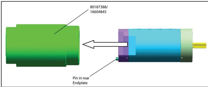
2. Thread Back Cap onto fixture. Tighten it to 40 nm (30 ft-lb) using a wrench.
