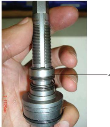
16. Grease collar spring, shutoff collar and spring guide with **Ingersoll Rand # 40036-1** grease in assembled condition.
