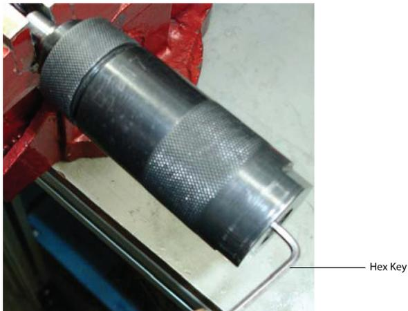
Remove Motor module from Motor Clamp Fixture 80187388 / 16604845.
