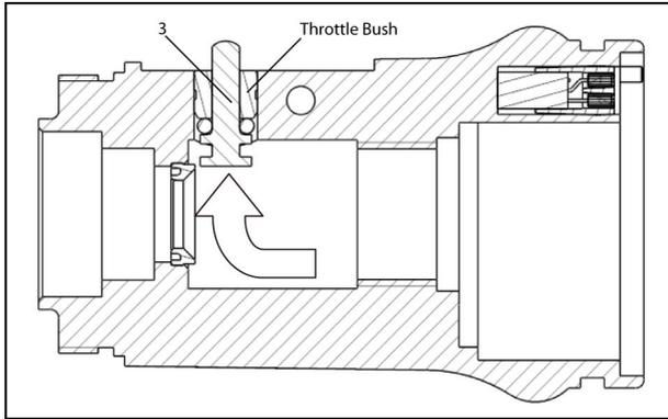
8. Insert ball (5) in Throttle Housing (1). Make sure, ball sits under Throttle Pin (3).
