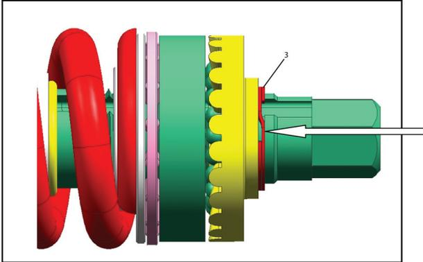
25. Grease unshielded side of Bearing (7) with **Ingersoll Rand # 68 Grease**.
