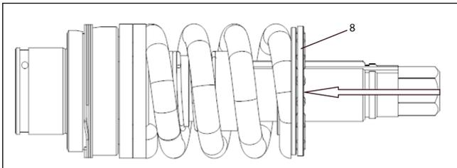
20. Slide Lock Nut Washer (17) onto above Assembly. Align Key on Lock Nut Washer with Keyway In Driver Shaft. See View Below for The Proper Placement.
