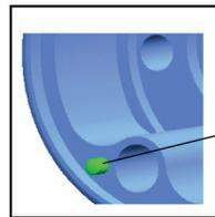
11. Grease Ball Spring (6) Ground Face and Mount on Inlet Bushing Assembly (12) Mounting Face.
