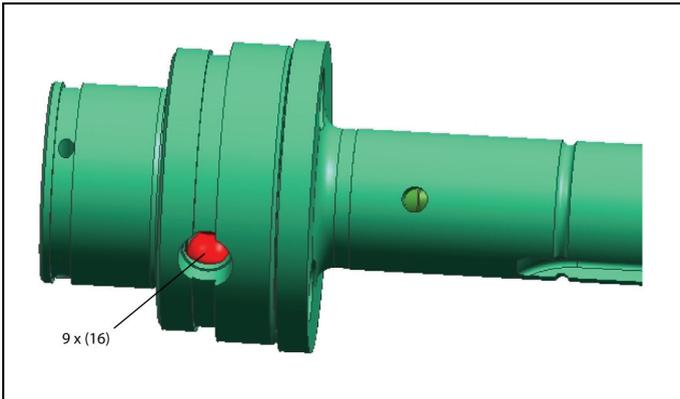
16. once all balls are removed, separate Driver Shaft (9) from Upper Driven Jaw (18).
