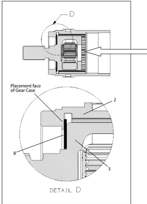
4. Grease Spindle Assembly's (3) gears with **Ingersoll Rand # 90 grease**.
