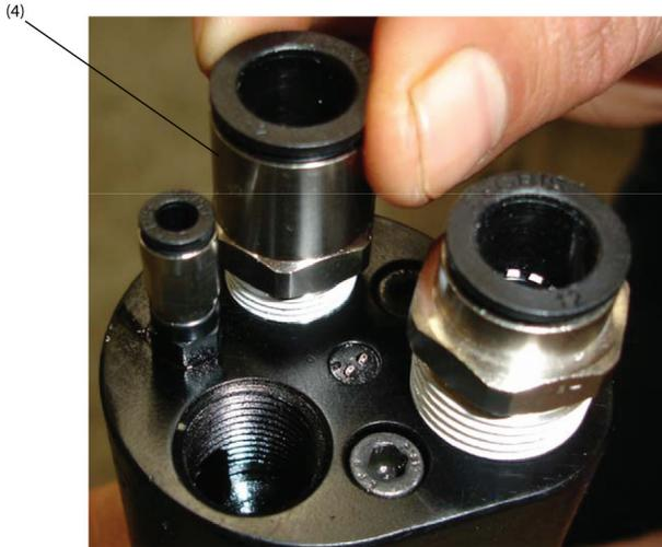
4. Tighten Tube fitting (4) onto Secondary exhaust hole threads in Remote Backend Housing using spanner wrench.
