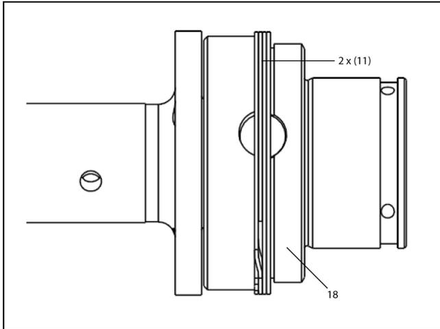
7. Grease Ball Pocket of Driver Shaft (9) with **Ingersoll Rand** 40036-1 Grease.
