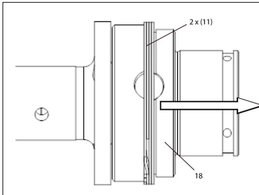
14. Remove Plug from driven jaw by tapping upper driven jaw gently against the work surface.
