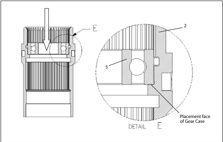
2. Grease Gear Case's (2) Splines with **Ingersoll Rand # 90 Grease**. Place Spindle Assembly (3) onto bearing in gear case with hand first and then press using manual press to butt against the placement face of bearing. Support bearing inner race during pressing. See section and detail views below for the placement.
