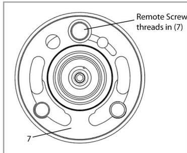
6. Insert Screw (9), Qty 2 in the counter holes in remote start housing of above assembly and tighten screws onto screw's threads in remote motor housing by hand first.
