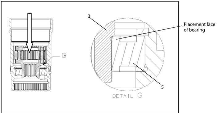
4. Grease Spindle Assembly's (3) Gears with **Ingersoll Rand # 90 Grease**.
