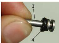
7. Install throttle pin (3) with O-ring in throttle housing (1) using needle nose pliers. Adjust to get throttle pin into throttle bush. Throttle pin must be visible from outside over throttle housing bush area.
