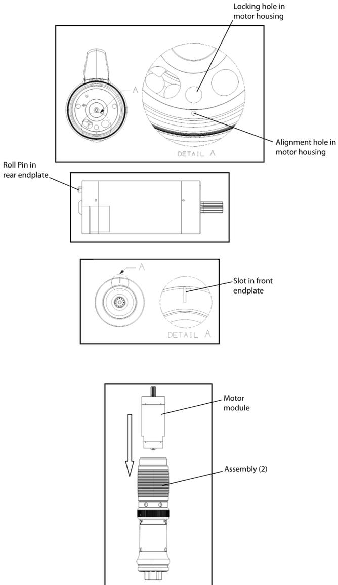
**Note:** Make sure that the roll pin in the rear endplate of motor module goes into the locking hole in motor housing of assembly (b).
