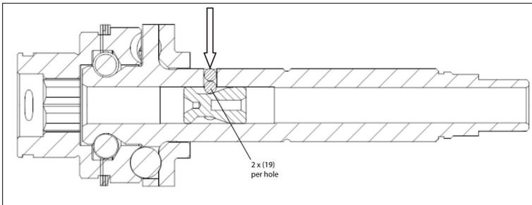
12. Grease I.D of shutoff collar (13) with **Ingersoll Rand # 40036-1 Grease**. Slip shutoff collar over drive shaft.
