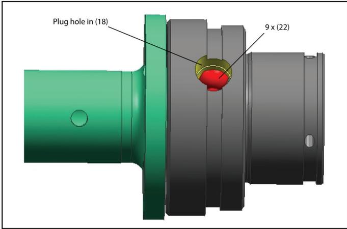
5. Place Plug (16) in plug hole of upper driven jaw (18). The smaller diameter of plug must face ball (22) inserted in step (3)
