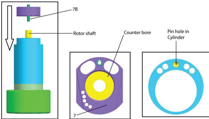
9. Grease Bearing (5) with **Ingersoll Rand # 68 Grease** and place onto Rotor Shaft and Rear Endplate Assembly counter Bore. Press Bearing Using Fixture 80187370 Until Assembly is tight and will not rotate.
