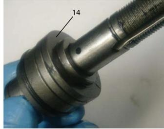
10. Grease Plunger's (12) outer surface with **Ingersoll Rand # 40036-1** Grease. Insert Plunger Into Driver Shaft's (9) Hole through upper driven jaw's hole. See section view below for the proper placement.
