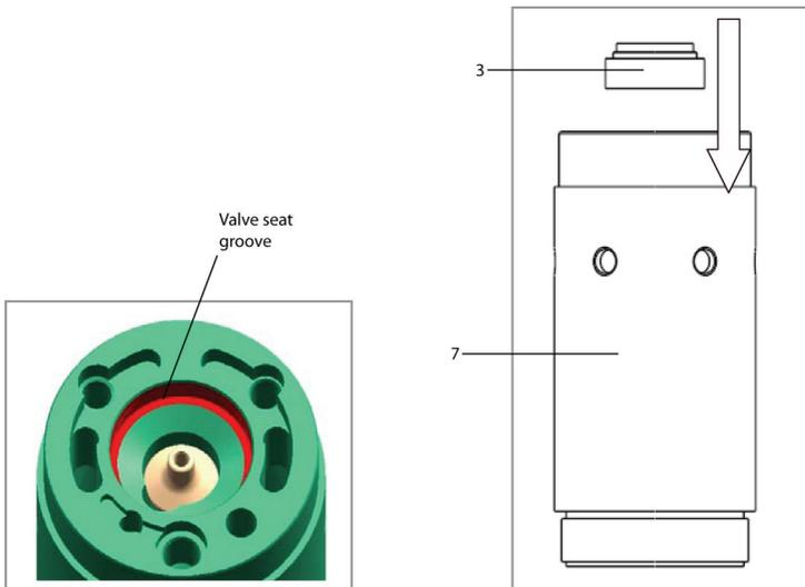
2. Grease O-ring (4) with **Ingersoll Rand # 68 Grease** and Mount on the Valve Seat's (3) O-ring Groove in above Assembly.
