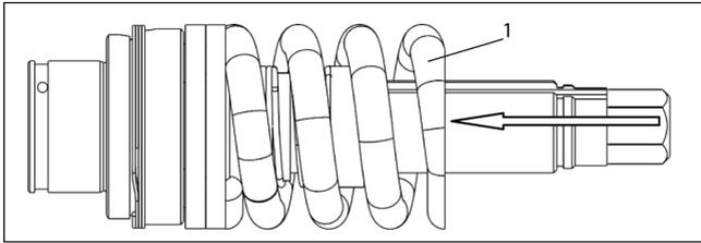
18. Grease both faces of spring guide (15) with **Ingersoll Rand # 40036-1** grease and place over clutch spring (1).
