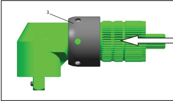
2. Place Coupling Nut Retainer (4) on the groove of angle housing of above assembly by using heavy duty retaining ring pliers.
