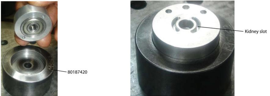
5. Place Rotor onto front endplate bore. Hold fixture 80187370 in manual press and press rotor in front endplate.
