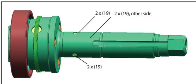
9. Remove Retaining Ring (Qa8-701) from upper driven jaw's (18) retaining ring groove.
