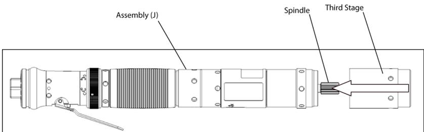
2. Mount Spacer (QA8-208) in Gear case (QA8-31-37) of the Third stage assembly (QA8-M37-4P29-1) for QAAA..150.. and QAAS..090.. models.
