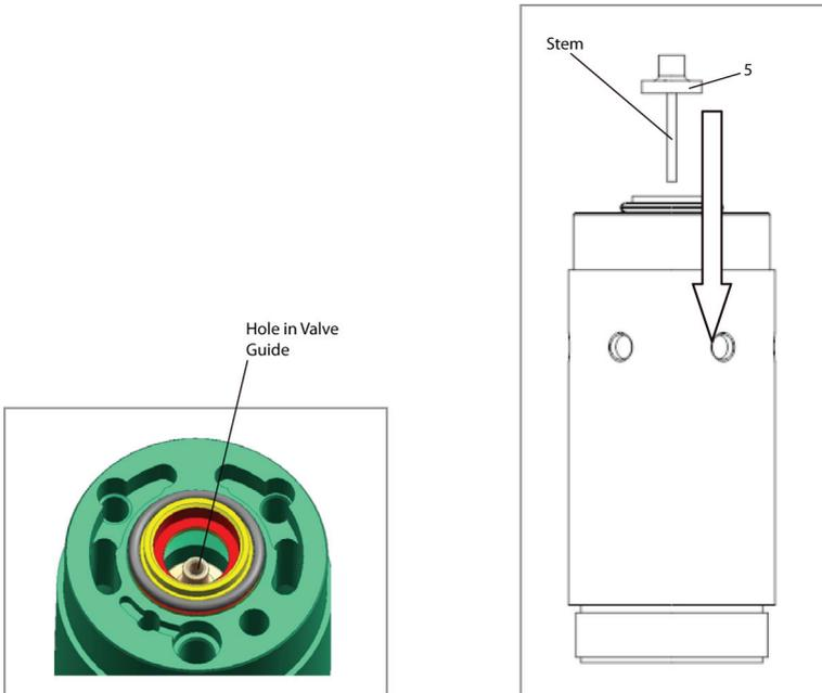
4. Grease O-ring (6) with **Ingersoll Rand # 68 Grease** and Mount in Remote Start Housing (1) Internal Groove.
