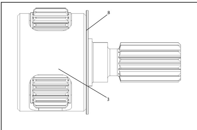
3. Grease Gear Case's (2) Splines with **Ingersoll Rand # 90 Grease**. Place The above Assembly ( I.e Spindle Assembly and Spacer) In Gear Case (2). Spacer (8) Mounted on Spindle Assembly Must Butt Against The Placement Face of Gear Case. See Section View for The Proper Placement.
