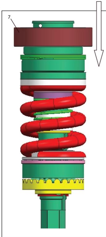
**Note:** Assemble Push Rod (6), Sun, Pin (Qa6-15) and Retaining Ring (Qa8-701) During Assembly of Complete tool.
