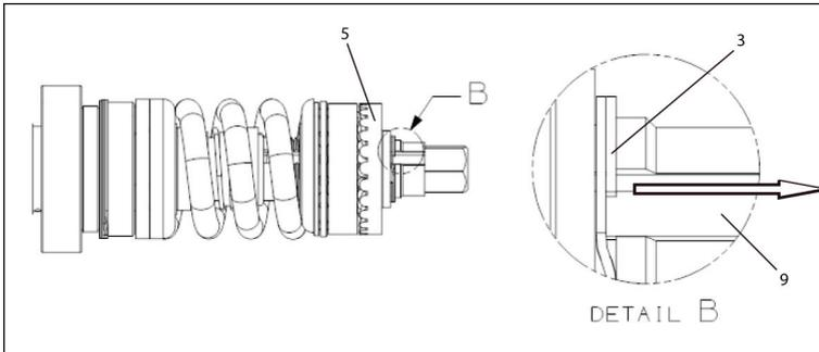
2. Insert The Bit of torx Driver (125116) in the teeth of Adjustment Nut (5) and Nut Lock Washer's (17) Slot. Rotate torx Driver in Clockwise Direction to loose Adjustment Nut.
