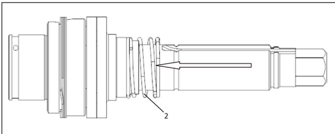
14. Slip Spring Guide (10) over Drive Shaft. The Other Flat Face of Collar Spring must sit on the step of Spring Guide.
