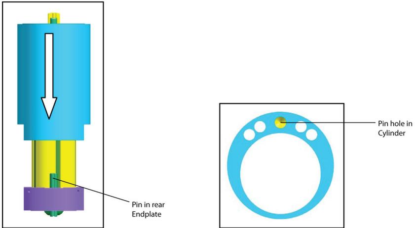
5. Place Front Endplate (with Wave Washer and Bearing) assembly onto rotor shaft. Align roll pin (8b) in cylinder assembly with pin hole in front endplate.
