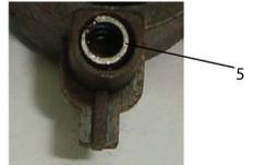
5. Coat O-ring (4) with o-ring lube and place on the groove in reverse valve (3).
