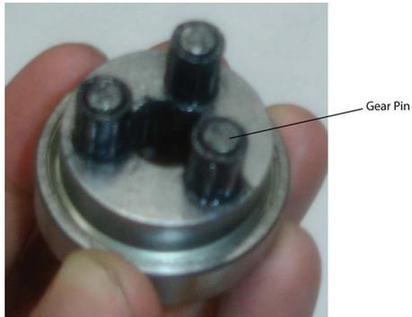
2. Place Planet Gear, Qty # 3 onto Needle Roller Bearings of above Assembly.
