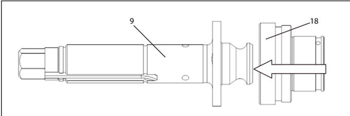
4. Grease 9 X Ball (22) with **Ingersoll Rand # 40036-1 Grease**. Insert them one by one in the Ball Groove of Driver Shaft (9) and upper driven jaw (18) through plug hole of upper driven jaw.
