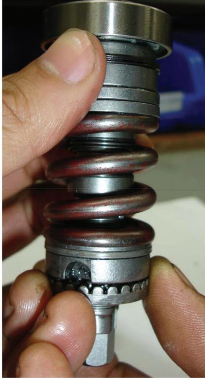
4. Remove Nut Lock Washer (17), Bearing (8), Spring Guide (15) and Clutch Spring (1).
