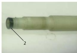
3. Press Ball Seat (2) with Ball Seat Assembly tool into Throttle Housing by using manual press. See Section view for the proper placement.
