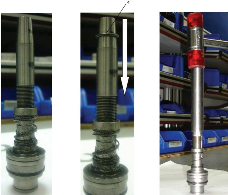
**Note:** 1. Check That Retaining Ring (4) is Correctly Positioned onto Driver Shaft's (9) Groove. 2. Make Sure that the Plunger Positioned in Steps 10 and 11 is in its Position.
