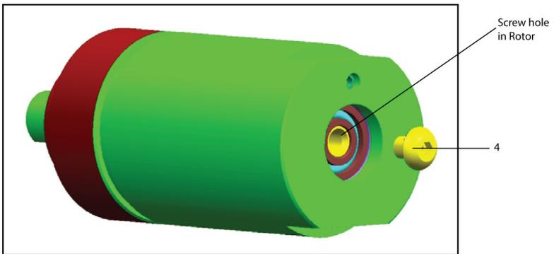
5. Slowly tighten Adjustment Screw. Tighten it until Assembly rotates freely.
