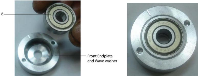
4. Place above assembly in the counter bore of fixture 80187420. Kidney slot side of front endplate must be upward.
