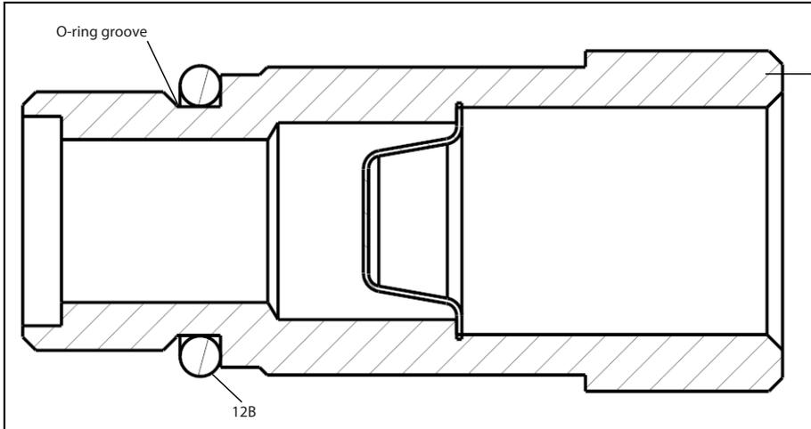
2. Coat o-ring (12B) with o-ring lube and mount on inlet bushing (12A) O-ring groove. See section view for the proper placement.
