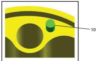
5. Put chip holder assembly (11) into Chip holder assembly hole in throttle housing (1) so that leads are showing.
