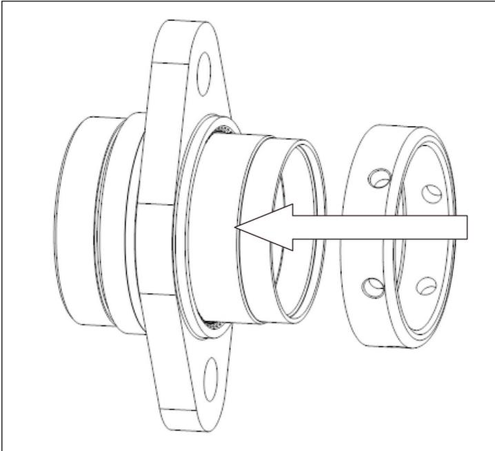
3. Grease Bearing (3) with **Ingersoll Rand # 68 Grease**.
