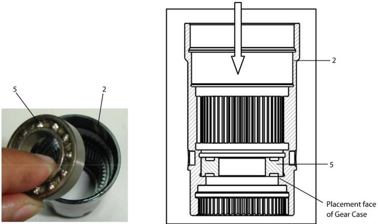
2. Secure Bearing (5) with Retaining Ring (4) using internal circlip pliers. See section and detail views below for the proper placement.
