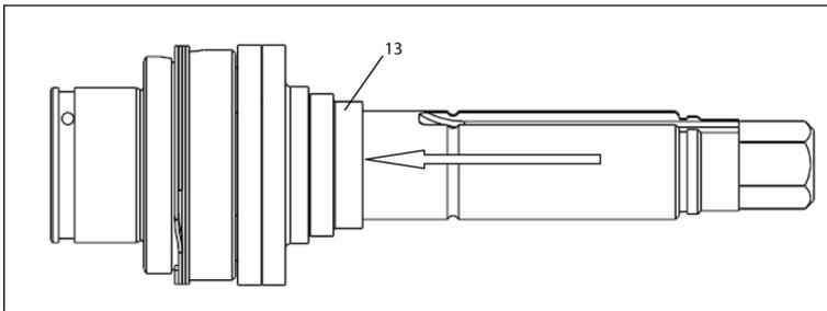
13. Slip Collar Spring (2) over Drive Shaft. Flat face of Collar Spring Must Sit on the Step of Shutoff Collar.
