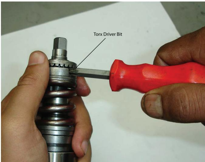
3. Rotate Adjustment Nut in counter clockwise direction to remove.
