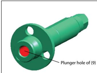
3. Insert Upper Driven Jaw (18) onto Driver Shaft (9).
