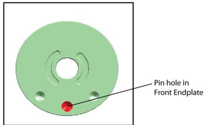
8. Put Rear Endplate Assembly onto rotor shaft. Align roll pin (7B) in rear endplate assembly with cylinder pin hole.
