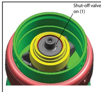
4. Grease O-ring (3) with **Ingersoll Rand # 68 Grease**. Mount It over The O-ring Groove (External) of Valve Seat (1) of above Assembly.
