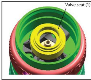
3. Place Shut-off Valve (4) on the shut-off valve groove of valve seat (1) of above assembly. Make sure that stem of shut-off valve passes through the hole in valve guide in motor housing.
