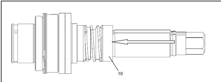
15. Use Retaining Ring tool (80187362) to place Retaining Ring (4) on Driver Shaft (9) Groove.
