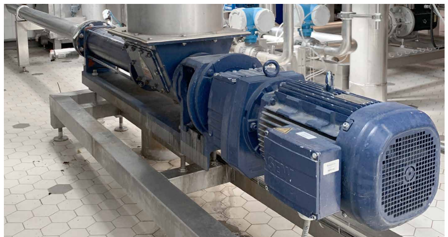
The hopper of the BTQ 35-12 can be easily cleaned thanks to inspection flaps on both sides.
