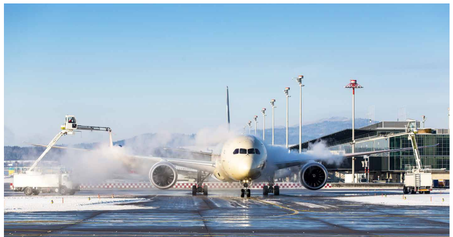
De-icing of an airplane wing just before take-off.
