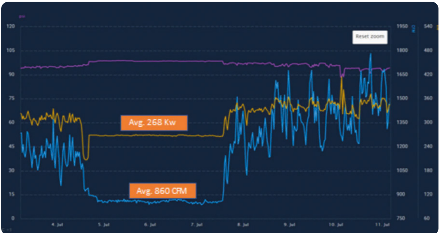
Figure 2: Non-productive air flow measured during plant shutdown
