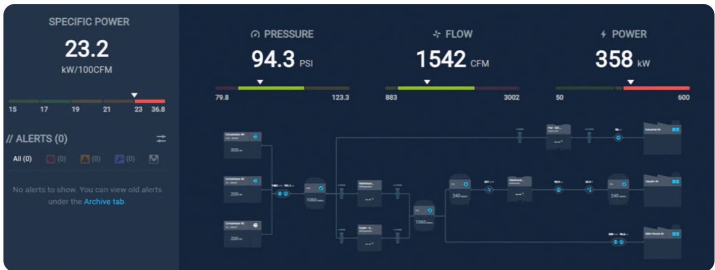
Figure 1: Compressed air system live P&ID dashboard
